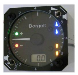
All basic **total energy variometer/audio** functions and ALL the advanced variometer functions of **digital averager, integrator, comparator, speed command, netto/relative netto and speed command audio**, with all functions properly altitude compensated to 22,000ft (6,700m) and serial data output including GPS, air data and pilot settings.
