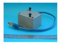
A small high performance 16 channel GPS unit is an optional part of the B800 and plugs in to a connector at the rear of the B800. This GPS uses the latest low power technology and draws less than 30mA at 12 volts as well as providing genuine 4Hz (4 times a second) fixes.
