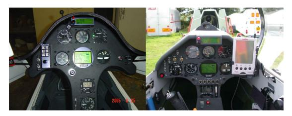
Photos of installations in a Discus 2 and an ASW27B. Note these are early B500 instruments with red push buttons(now black).
