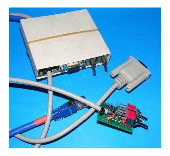
This optional device connects to the B800/B500 or other variometer system and supplies power and data to various other devices - a B2500 glide computer, a Flight Recorder(FR), a Flarm unit(or second FR) and a PDA/PNA which can receive 5 volt power at 1 amp and data from the B800.
